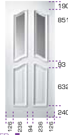
COSMOPOLITAN GLAZED Sash size. MAX 818 x 2005 MIN 726 x 1736 Frame size with Threshold. HxW. MAX 930 x 2083 MIN 838 x 1814
