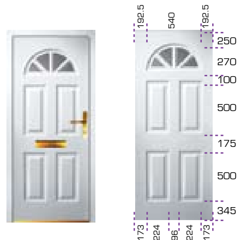
CAROLINA BEAD GEO BAR GLAZED Sash size. MAX 888 x 2098 MIN 744 x 1730 Frame size with Threshold. HxW. MAX 1000 x 2176 MIN 856 x 1866
